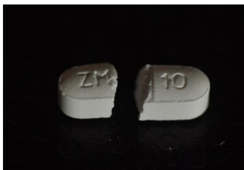
Figure 1. Tablet with titanium dioxide coating. Cut to allow identification of composition.
