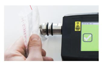
With the *point and shoot adapter* analysis can be made from any surface by gently pressing the adapter against it.
