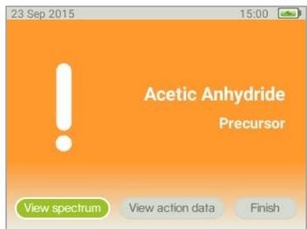
An orange screen is shown with the name of the substance found and a warning text indicating that this substance has been classified as a precursor, meaning that it may be used to manufacture a regulated substance (in the Screen category used for this measurement).
