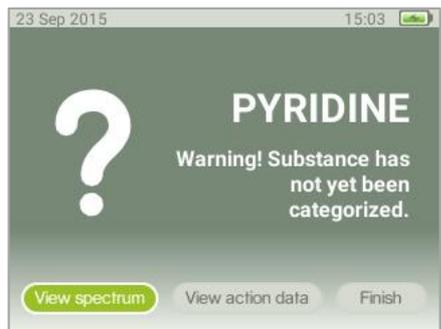
A gray screen is shown with the name of the substance found and a warning text indicating that this substance has not yet been categorized in the “Screen Category” selected for this measurement. As such, the instrument would not know if this is a regulated substance or if it belongs to any of the less severe categories.
