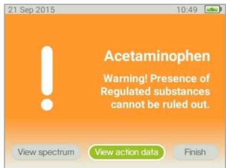
An orange screen is shown with the name of the substance found and a warning text indicating that this substance has been classified as a masking agent, meaning that it may be used to mask/hide the presence of a regulated substance in the sample.
