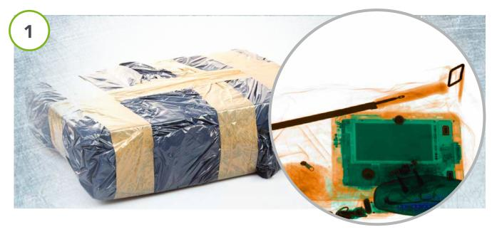
If suspect items (solids, liquids, powders) are found they are screened using Raman spectroscopy. In the case of explosive materials, the facility's bomb threat procedures are put into effect. Measurement data is stored in ChemDash for later reference.
